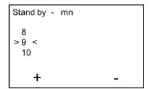
When the Dualex enters the standby mode, all measurements and settings are saved. When you restart the device by a long press on the button , to measure, a new self-calibration is needed.
