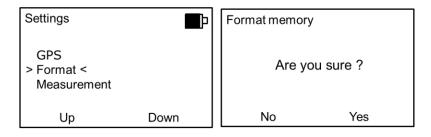
If the buttons (No) or are selected, the data are left intact and the software returns to the main menu.
