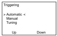
Automatic (by default): at every closure of the clip or a press on the button , a measurement is saved.
