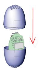
D: Pressed and rotate clockwise to close.
