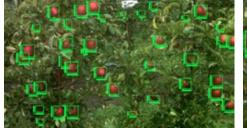
Tele lens focusing on a tree and detecting the apples automatically (CropVIEW<sup>®</sup> automatic detection).
