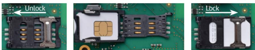
3. Slide the metal part of the SIM card holder to unlock it. 4. Place the SIM card into the holder so the gold contacts on the SIM face down on the board. 5. Lock the holder by sliding the metal lock.
