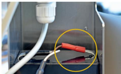
6. Connect the red cable to the positive battery terminal.
