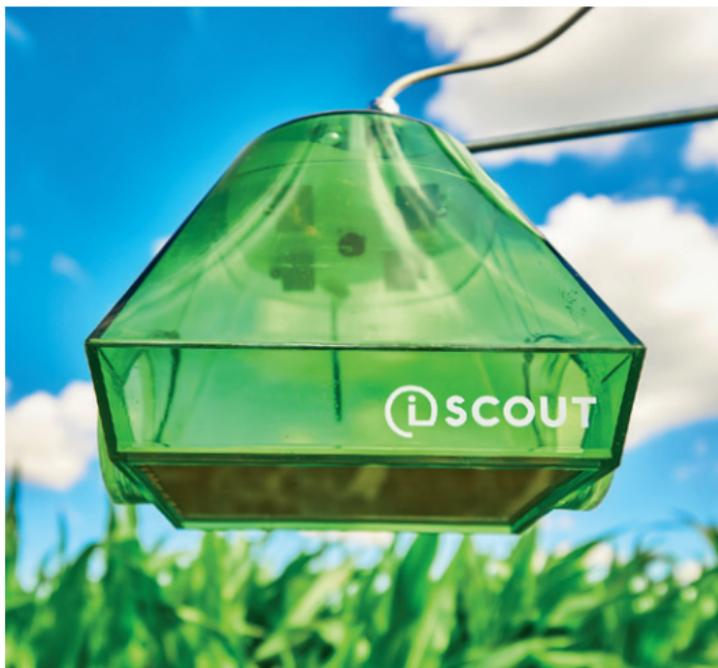
Thank you for choosing iMETOS iSCOUT® for Remote Trap Image Monitoring. iMETOS iSCOUT® periodically takes high resolution photos from the insect trap. Photos are automatically uploaded to the FieldClimate platform without the need of any user intervention, thus allowing a continuous insect control in the agricultural sector.
