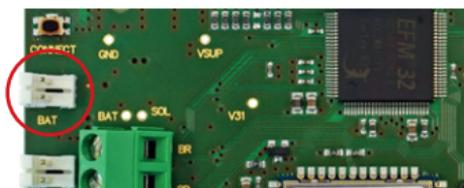
Plug the battery cable into the BAT connector on the PCB (red circle).
