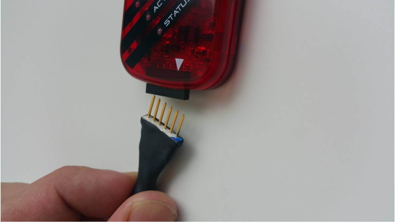
Picture 2 - connecting the programming cable to the Microchip PICkit3 programmer
