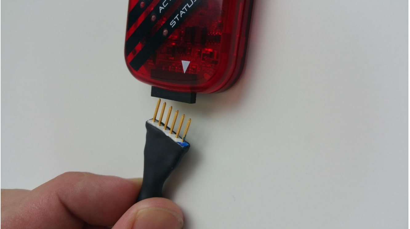
Picture 4 - connecting the programming cable to the Microchip PICkit3 programmer
